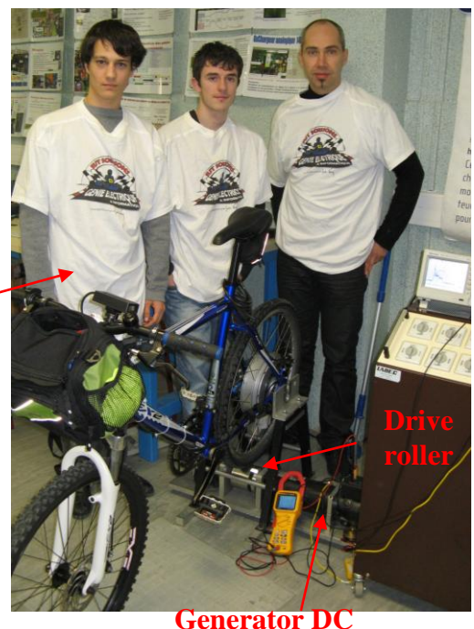
Figure 4 : elec bike and testbed
